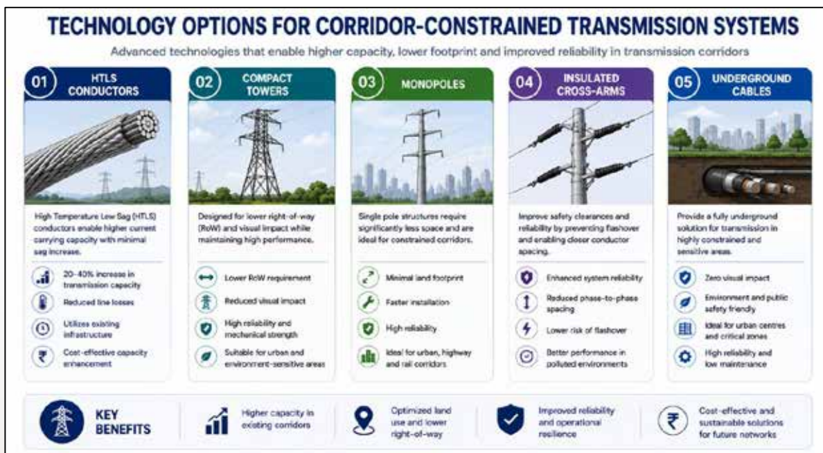
Figure 29: Technology Options for Corridor-Constrained Transmission Systems
